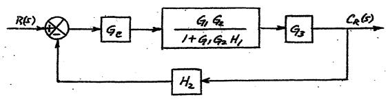
The closed-loop transfer function  $C_R(s)/R(s)$  can be given by
